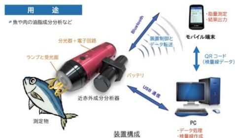
Fig. 7 Measurement of fat content in fish
