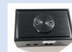
Light source for checking photon counters
